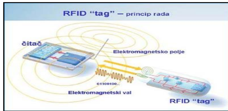
Figure 3. Working principle of RFID "tag"
